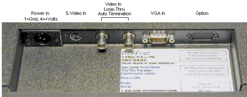
Monitor Backside, Connector Well Area, 15.1" Monitor. (Picture also shows VGA connector used on some models)
