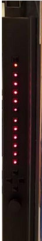
4. When the LEDs stop flashing, the routine is finished. Check monitor with a black screen. You can turn the brightness up to see the darkest areas of the picture. (Brightness quick access is to push the knob about twice without using the Menu button until the box appears at the bottom of the screen and says "Brightness". Then turn the knob up and down to inspect.)
