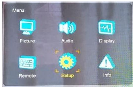
2. Rotate the knob until the Setup Icon is highlighted as above and push the knob. Next rotate the knob down to the Control line, push knob, rotate up (or down) to the Power Off/Screen Refresh line, push the knob, rotate to On and push again to choose. Use the left arrow key to back out of the Menu system. Next time you turn the monitor Off, the routine will now run, but only one time.
